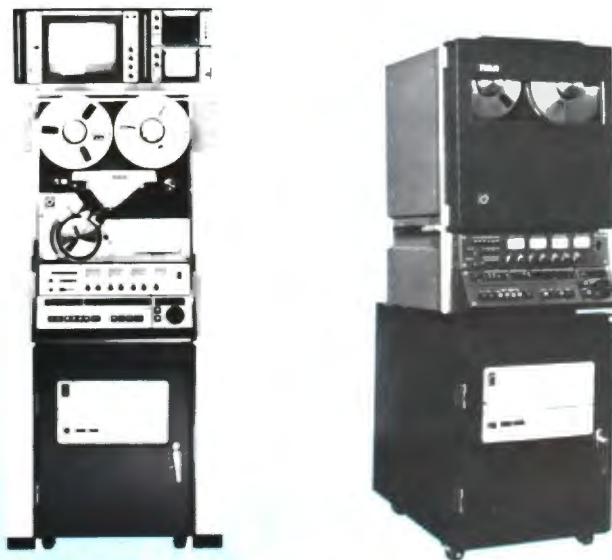
Console and T-cart mounting configurations
