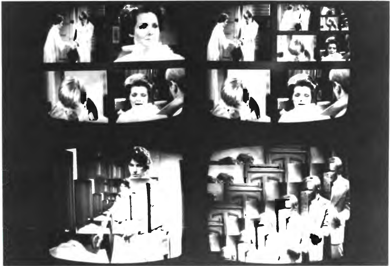
Visual Effects: The dual freeze feature enables the TFS-121 to display up to four compressed frozen pictures in any of the four raster quadrants (upper left). The freeze quadrant also can be moved to any of the other three quadrants (upper right). A hall of mirrors effect is achieved by keying the output of the synchronizer back on itself (lower left and right).
