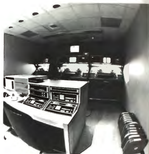
Post-production tape editing suite. With expanded production requirements, four TR-600A VTR's with AE-600 editing systems have been added.
