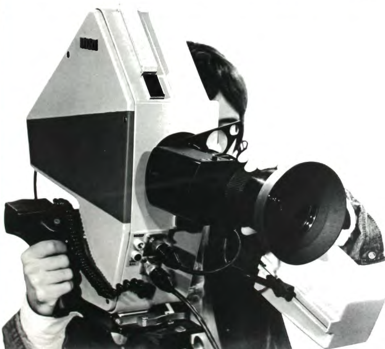
Studio camera conversion using Minimax adaptor
