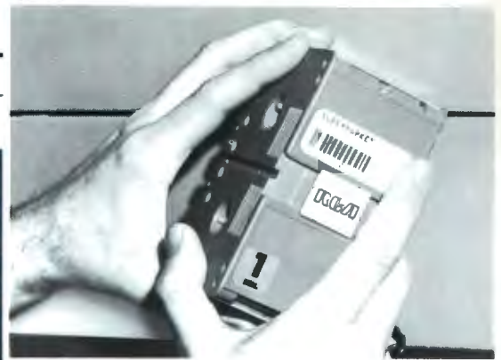
TCR-100A cartridge with Bar Code label for optical readout.
