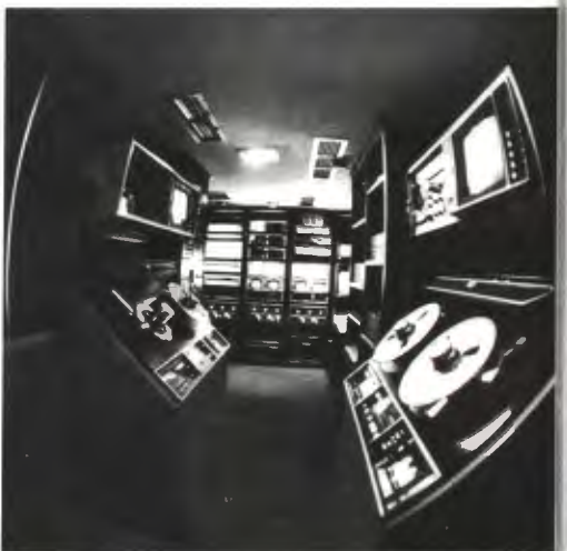
Inside PTL's 45-foot van is a complete studio. Two TR-600A tape machines with AE-600 editing systems; three TK-44's and a TK-76 are part of the flexible mobile unit.
