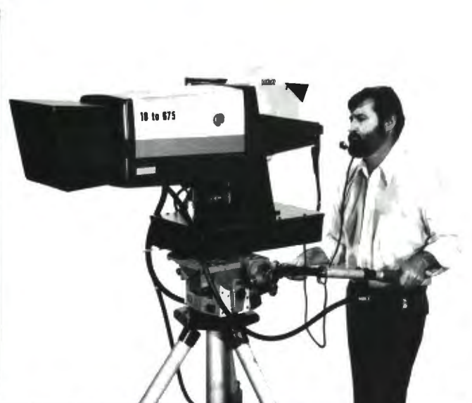
Studio camera conversion using Minimax adaptor
